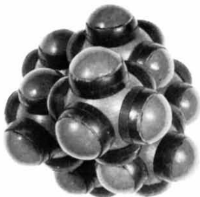
Fig. 15. Rhombohedral R\bar{3} structure simulating the crystal structure of WCl_6 (Model 14).
