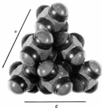
Fig. 12. Monoclinic C2/c structure simulating the crystal structure of \alpha-CF_4 (Model 11).
